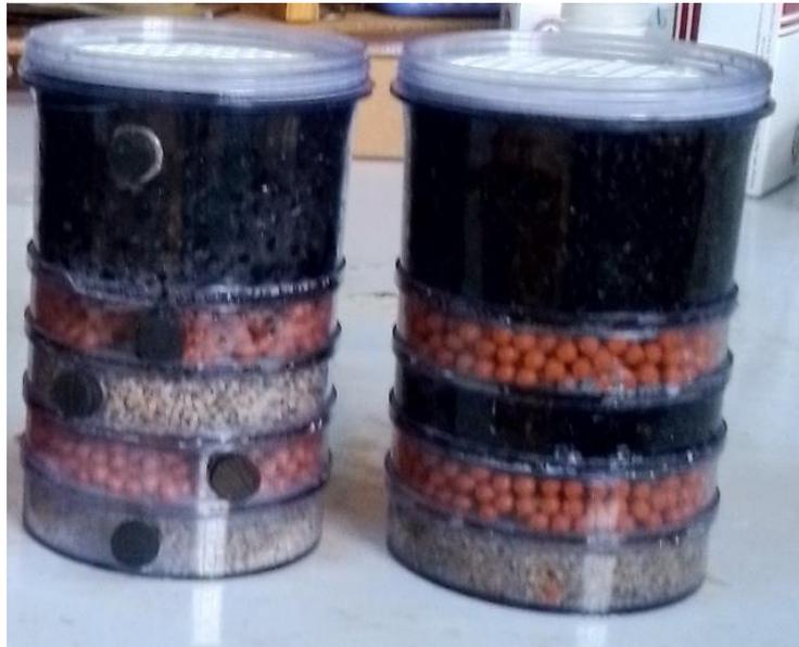
Figure 6. Constructed filter cartridge configurations
