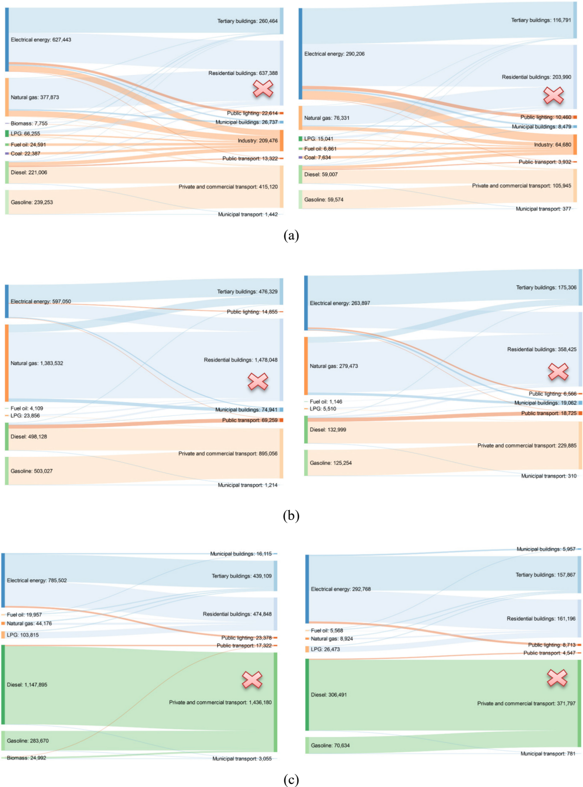
Figure 13. Sankey diagrams for energy (left, MWh) and CO 2 emissions (right, tonnes) for Messina (a), Trieste (b), and Cartagena (c); based on data in [63], [66] and [55]
