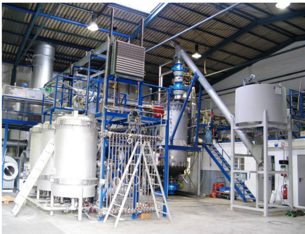
Figure 1. Photo of the pilot facility; from left to right: cracker, reactor, biomass bin
