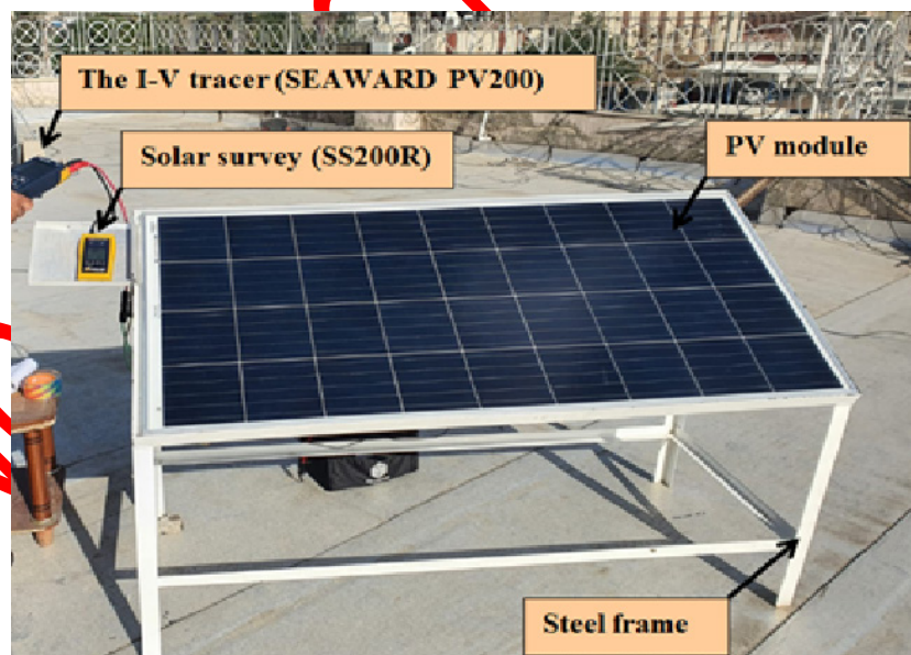
Figure 1. Tested PV module of nominal power 165 W
