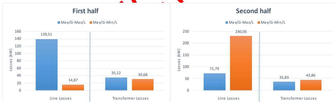
Figure 13. Line & Transformer Losses for different scenarios (Solar PVs installed in the first/second half length of the feeder)
