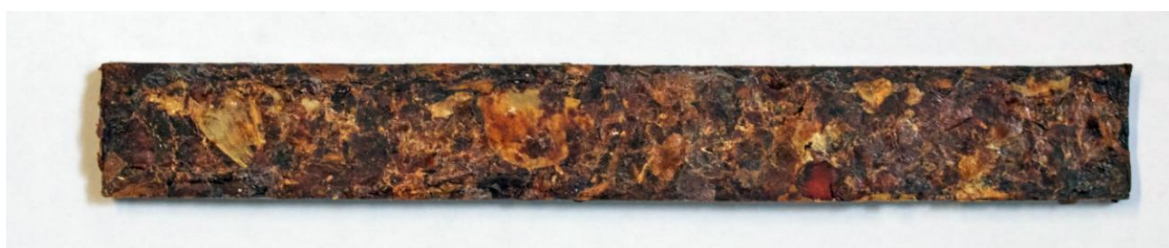
Figure 16. Briquetted sample of solid fuel obtained from apple pomace
