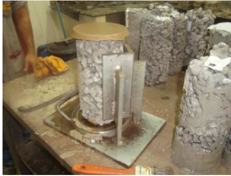
Figure 7. Capping of the upper and lower surfaces of the specimens
