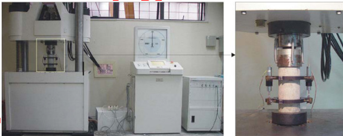
Figure 6. Servo-controlled Shimadzu, to perform the tests of resistance to axial compression
