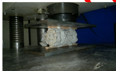
Figure 8. Test specimen positioned in the press, to perform the diametrical compression test.
