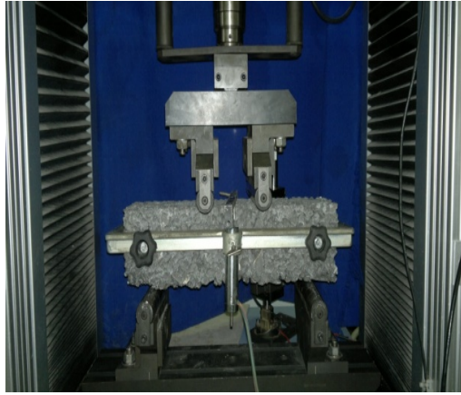
Figure 10. Positioning of the specimen for the flexural tensile test.
