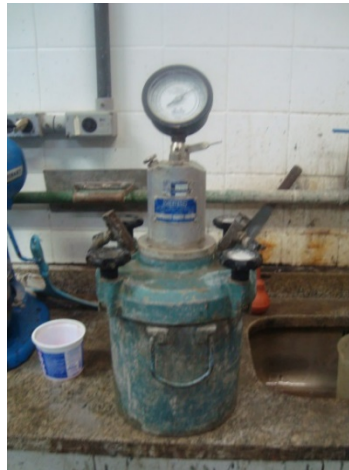
Figure 4. Built-in air meter
