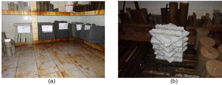
Figure 13. Curing of recycled concrete plates (a) and concrete plates
