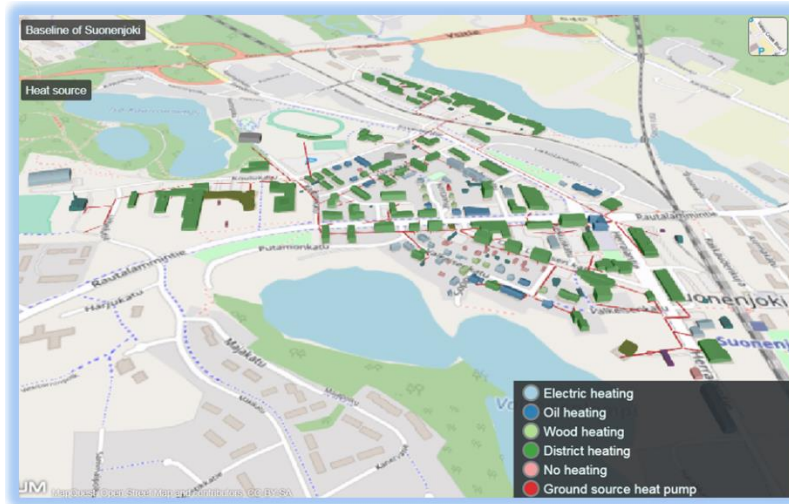
Figure 4. Schematic diagram of Suonenjoki DH network and building stock
